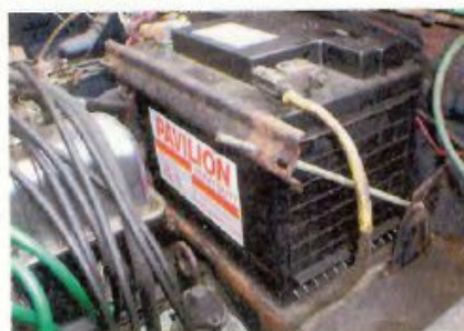
Remove battery if area around looks tatty – the metal tray below may well be rotten.
