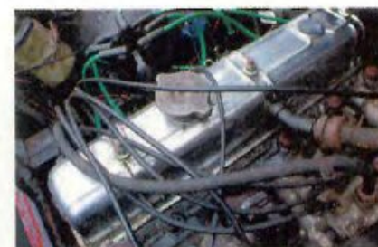
Sealing the engine is tricky. Check rocker and timing chain covers for signs of leaks.
