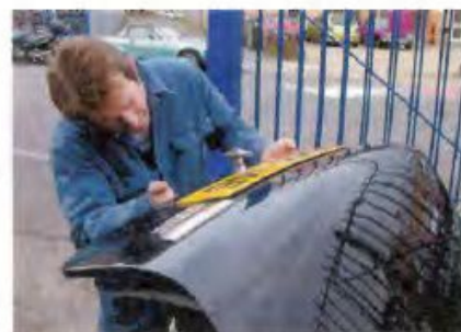
Trailing edge of the bootlid has a tendency to rot away allowing boot to fill with water.
