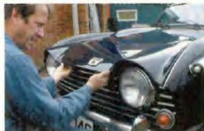
The front edge of the bonnet rots, and good replacements are tricky to find.
