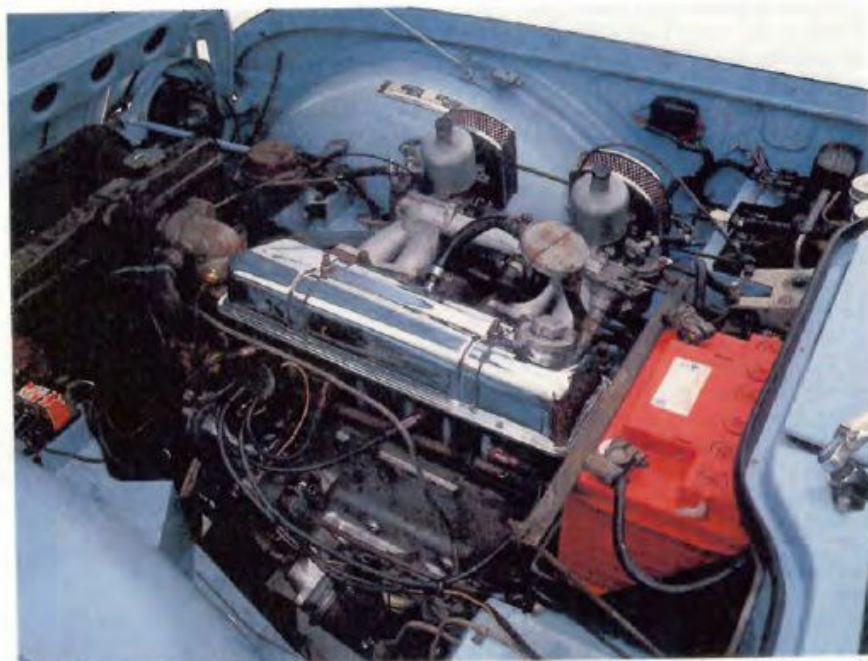
Four-cylinder 2138cc engine is torquey but not as sweet as TR5's six-cylinder 2498cc unit.
