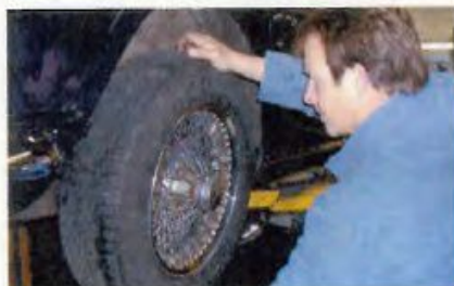
All four wheelbearings are prone to wear as they're under-engineered. Check for play.
