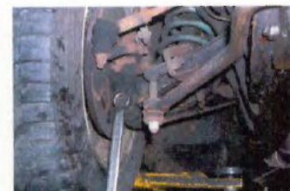
Unlubricated trunnions seize – this upsets handling and wears suspension prematurely.
