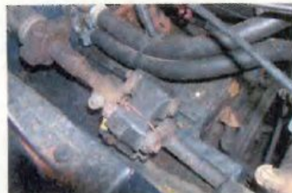
If the car's steering is vague or there's play, check doughnut above the bulkhead.
