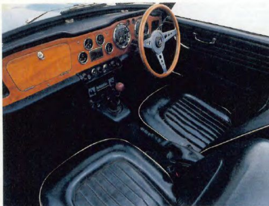
Typical British Sixties roadster has wooden dash, bucket seats and parts-bin switchgear.
