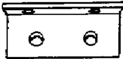
Slip the U-bolt over the column and through the bracket to check proper fit. then mark the firewall, drill two mounting holes and attach the bracket. Tighten the U-bolt, and your steering column should be free of the shakes from now on.
